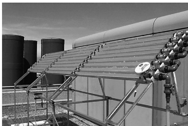
Fig. 1. View of the photoreactor used at the EPFL, Lausanne, Switzerland, compound parabolic collector (CPC).
